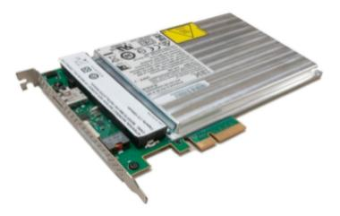
Figure 13.2 An IBM 4767 HSM as a PCI card. Photo from Wikipedia (http://mng.bz/XrAG).
